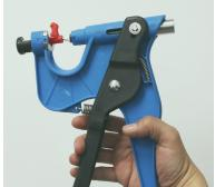
Rotate the black chamber to lock the punch into the device. Carefully squeeze the applicator handles together, guiding the punch tip into place if necessary. When the gun bolt rests flush against the red plastic clip, release the handle.
